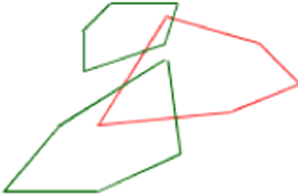
Fig. 8 Polygons obtained after projection in a ground plane. In this plane, the x-axis is oriented from right to left and the y-axis is oriented from bottom to up. The polygon in color green is from the first view and the polygon in color red is from the second view
